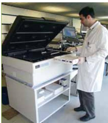
Figure I.16 - Measurement by liquid scintillation
