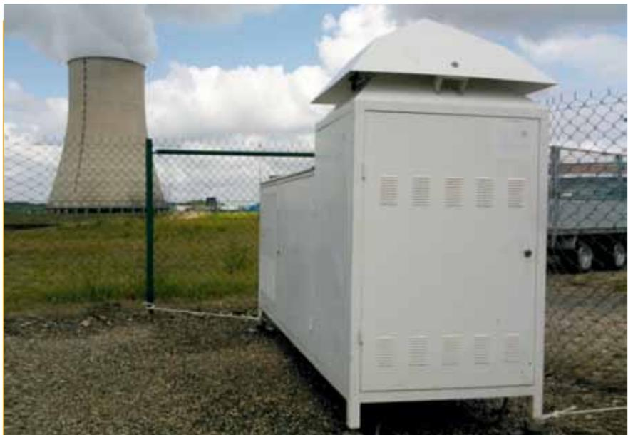
Figure IV.69 - OPERA-Air (300 m³/h) sampler installed under the prevailing winds of the Golfech NPP.
