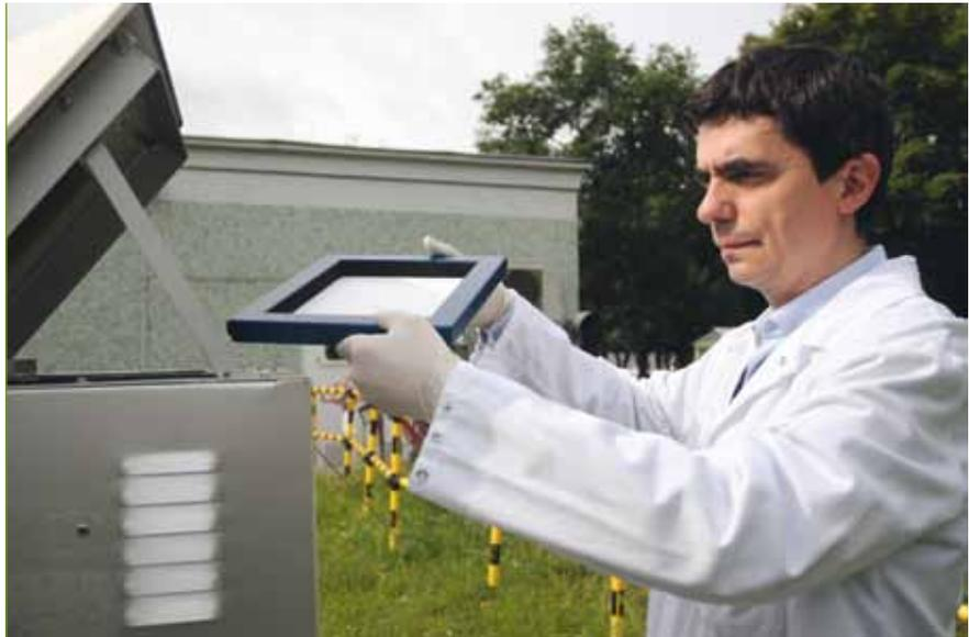
Figure 1.8 - Taking filter samples of atmospheric aerosols
