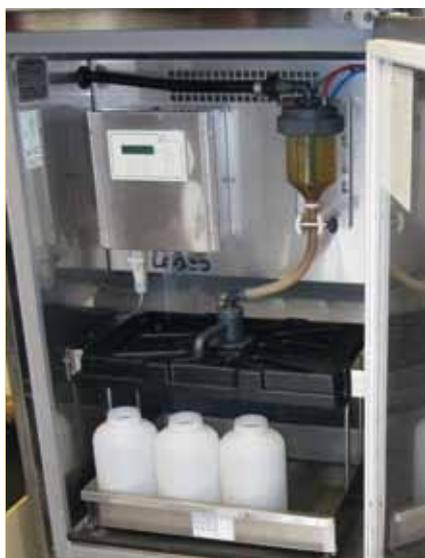
Figure IV.25 - Detailed view of an IRSN water sampler.
