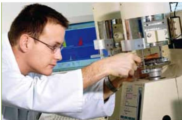
Figure I.15 - Alpha spectrometry measurement
