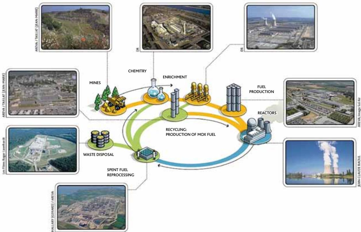
Figure 11.6 - Simplified illustration of the nuclear cycle
