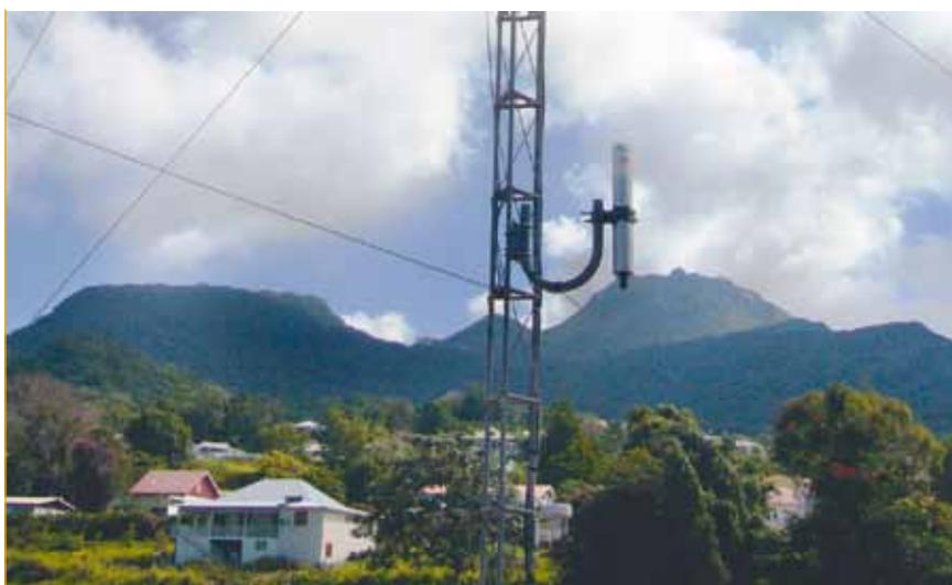
Figure IV.74 - New-generation Teleray probe installed in Saint-Claude, Guadeloupe.
