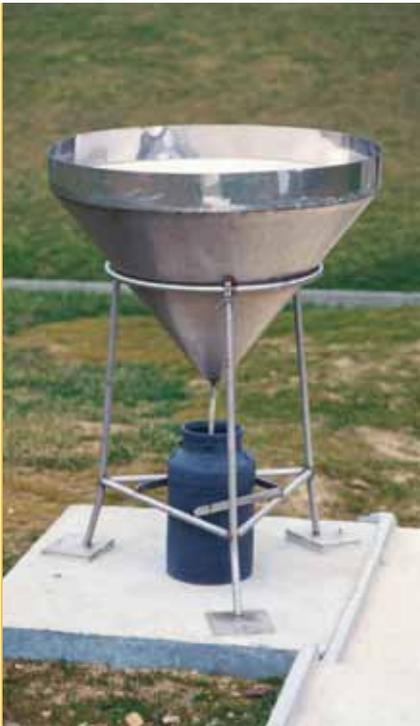
Figure IV.18 - Rainwater collector.
