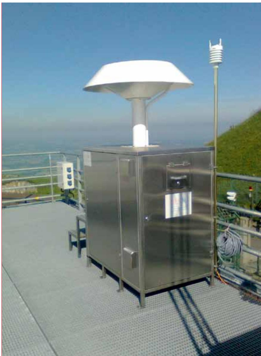
■ **Figure III.24** - Very high-volume (700 m<sup>3</sup>/h) aerosol sampler in IRSN's OPERA-Air network (Puy-de-Dôme site in south-central France).
