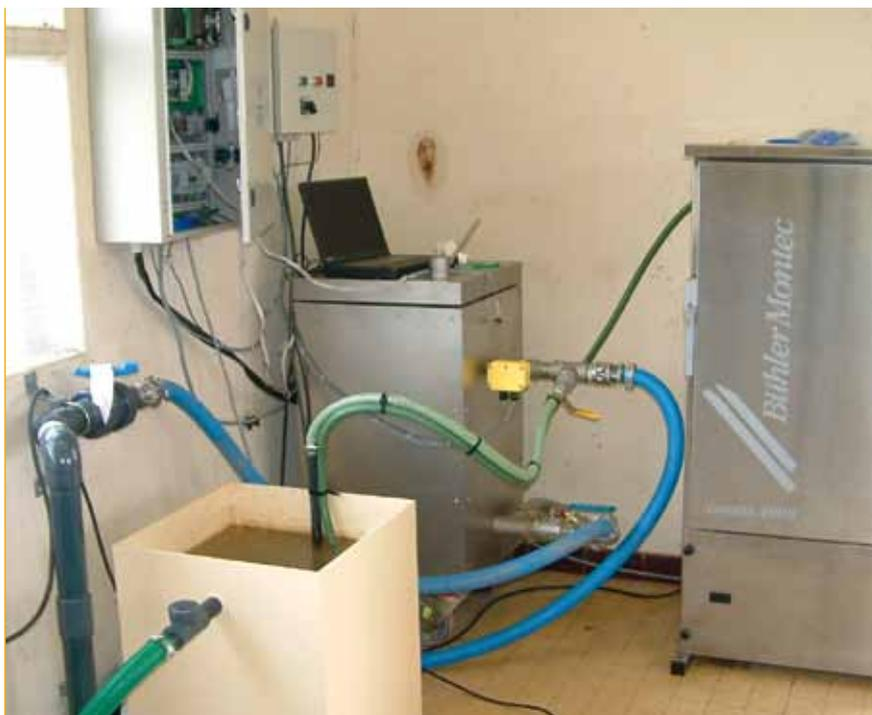
Figure IV.26 - Boé HydroTeleray station (near Agen) performing real-time radiological monitoring of water from the Garonne.
