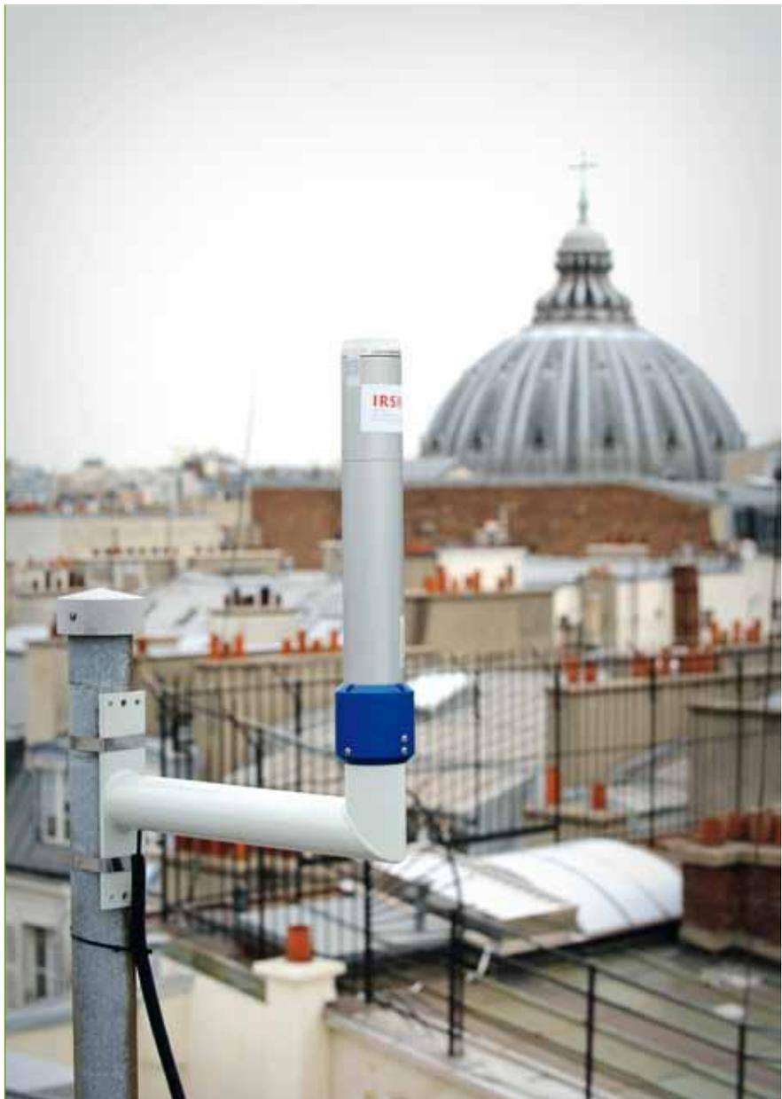
Figure 1.9 - New-generation IRSN Téléry monitor (for gamma radiation dose rate measurement) installed in Paris (French naval staff headquarters)
