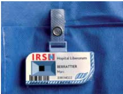
■ **Figure X.5 - Radio-photo-luminescent dosimeter.**
